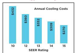
Annual costs based on 36,000 Btu unit, 1,500 cooling load hours, and .08/kwh. Actual costs may vary depending on climate conditions, energy rates and patterns of usage.
